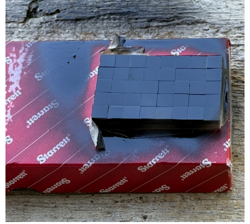
All inner surfaces of the Mass Density Cubes are painted with optically absorbent paint
